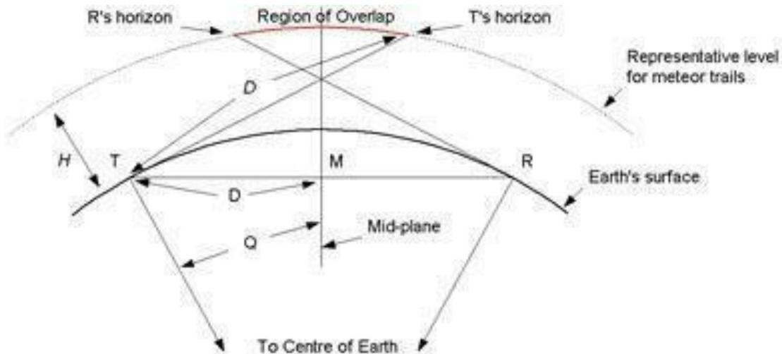
Based in the UK, we are fortunate to have a space-radar station at GRAVES, located just outside Dijon, France, which is ideally placed about 700km from central UK. This broadcasts at a frequency of 143.050Mhz.
